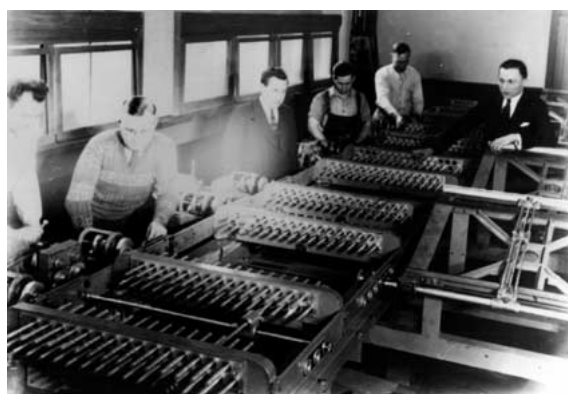
Figure 4. Mechanical computer, used by the author, with J.G. Brainerd, in 1939, to solve the non-linear differential equations representing enzyme-substrate kinetics at the Moore School of Engineering at the University of Pennsylvania.
