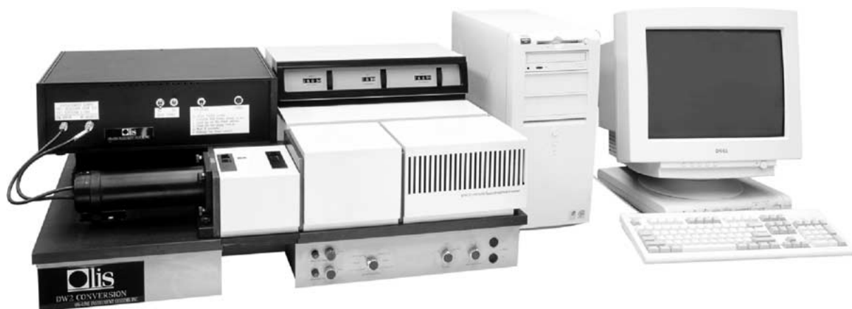
Figure 8. A photograph of the current version of a computerized dual-wavelength spectrophotometer (DW-2 Conversion). This photograph was provided by Julie DeSa Lorenz and John David Sturgill of Oils Company.
