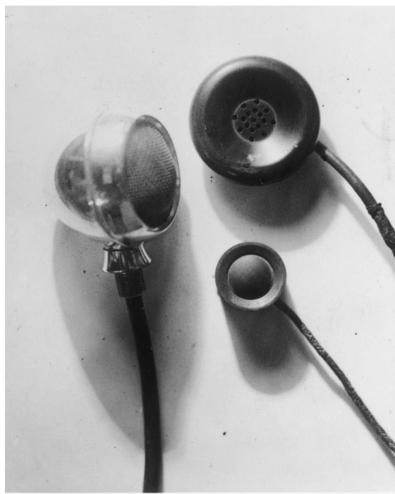
Figure 1. Top: Piezoelectric crystals of Rochelle salt. Lowest row shows cut wafers with electrodes attached. Bottom: Piezoelectric devices (microphone, earphone, stethoscope) Haifa, Fall, 1944.
