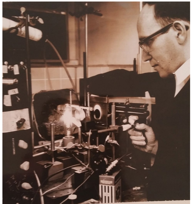
Fig. 8 Shmuel Malkin using a pistol to drive a high speed shutter in Bessel Kok's lab, ca. 1966
